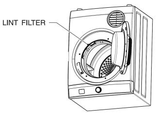
The lint filter is located at the front of your dryer at the top of the door opening.
